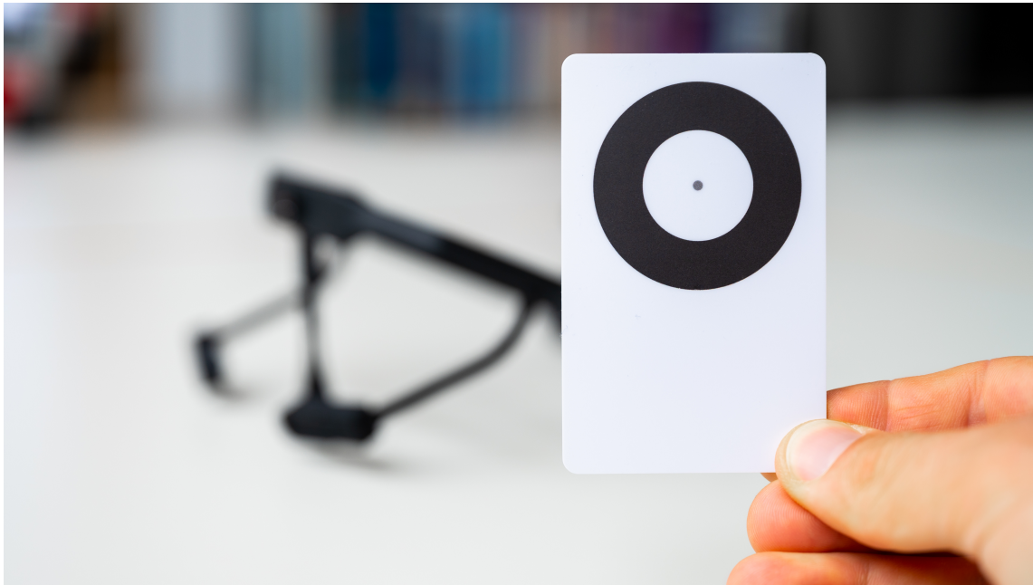
Fig. 2. Concentric calibration marker
